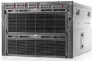
40 core Westmere EX @ 2.40GHz (Quad 10-core Intel® Xeon® E7-4870)
